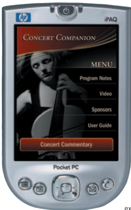
The Concert Companion, a wireless PDA, delivers concert commentary in real time.
